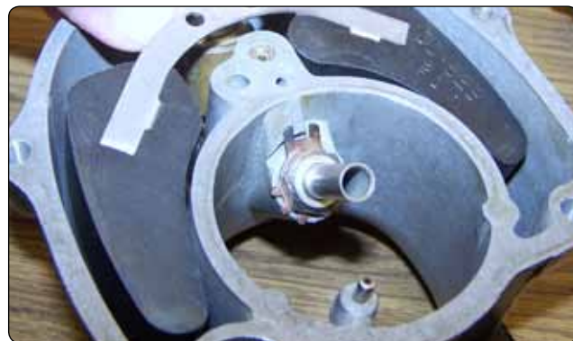
Figure 2-9. Float chamber discharge nozzle and float.
