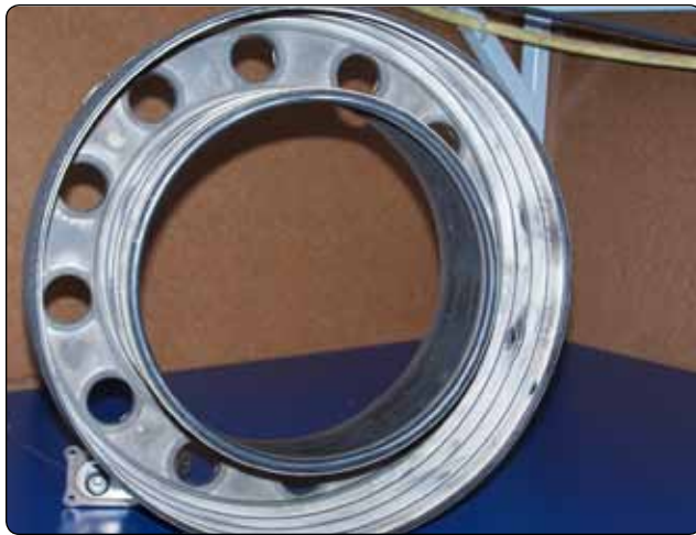
Figure 1-58. Annular combustion with chamber ceramic coating.
