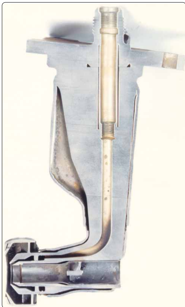
Figure 2-64. Simplex airblast nozzle cutaway.
