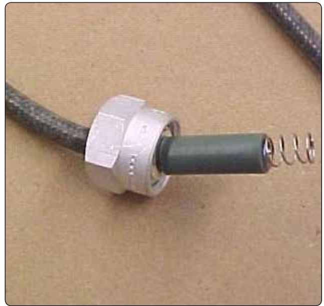
Figure 4-13. Ignition lead spark plug end.
