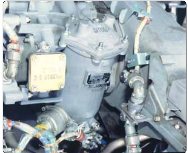
Figure 2-60. Dual element fuel pump.
