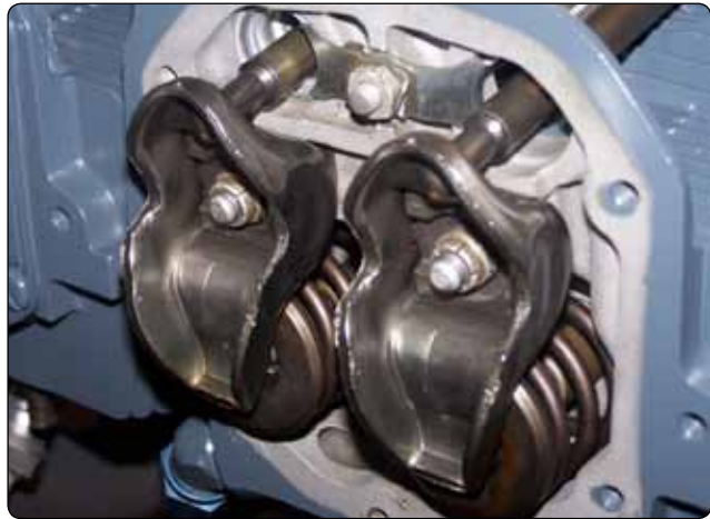
Figure 1-31. Rocker opposed engine arms.
