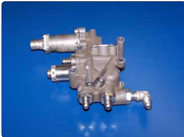
Figure 2-67. Flow divider.
