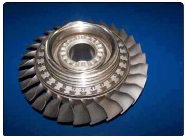
Figure 1-61. Turbine blades.
