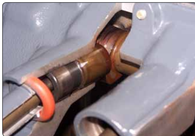
Figure 1-29. Cam load on lifter body.
