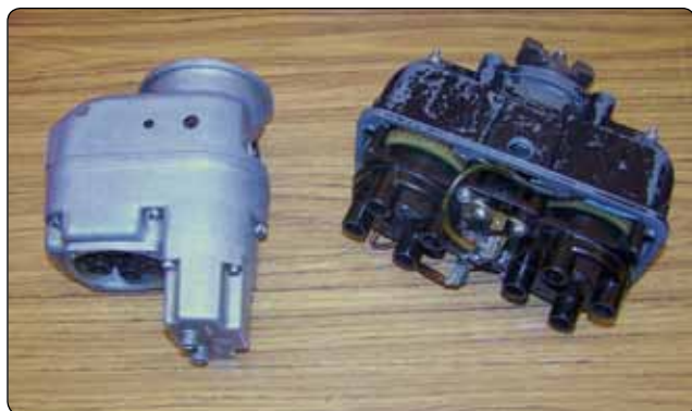
Figure 4-1. Single and dual magnetos.
