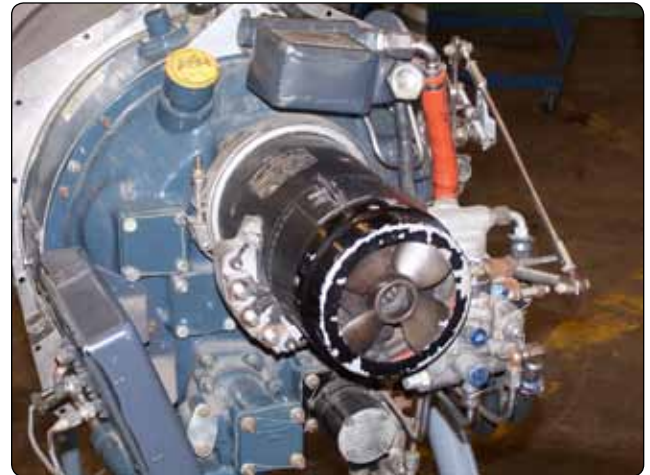
Figure 1-45. Typical turboprop accessory case.
