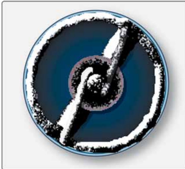
Figure 4-48. Carbon fouled spark plug.
