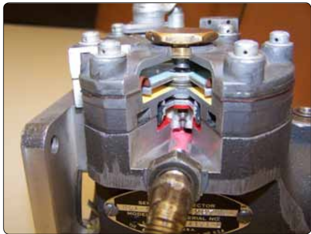
Figure 2-30. Cutaway view of airflow measuring section.
