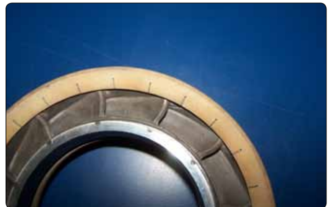
Figure 1-60. Turbine inlet guide vanes.
