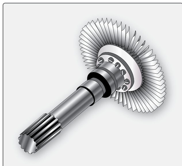
Figure 1-63. Rotor elements of the turbine assembly.
