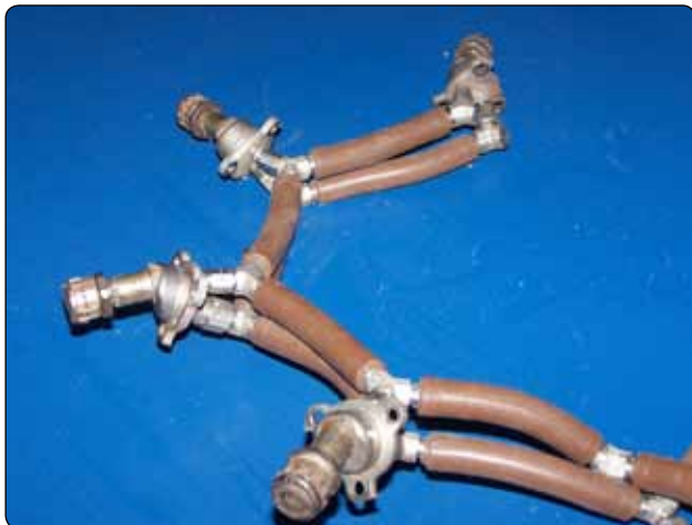
Figure 2-59. Fuel manifolds.
