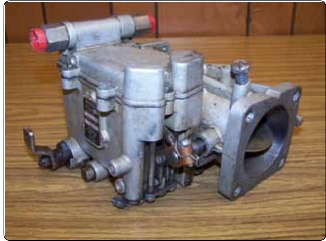
Figure 2-5. Side draft horizontal flow carburetor.
