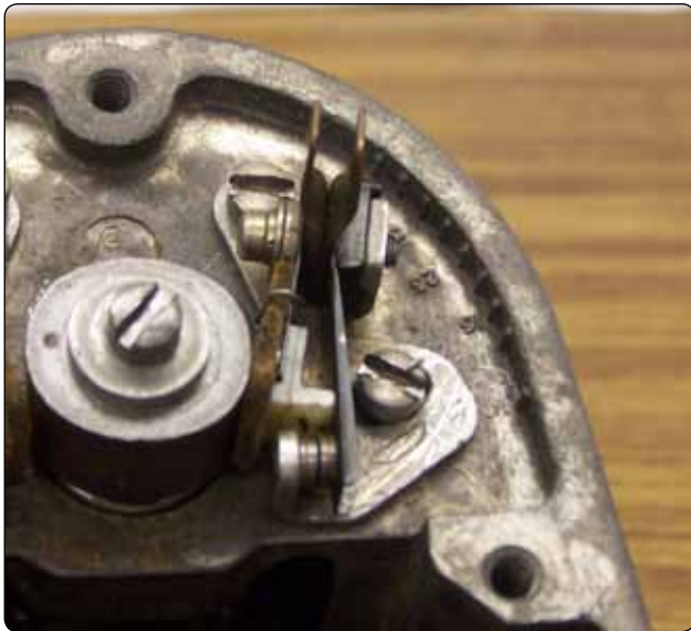
Figure 4-8. Pivotless type breaker assembly and cam.
