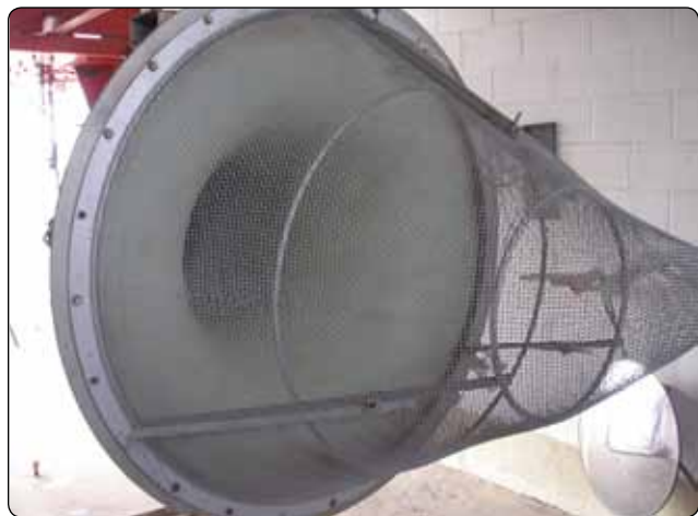
Figure 3-30. A bellmouth inlet used during system tests.
