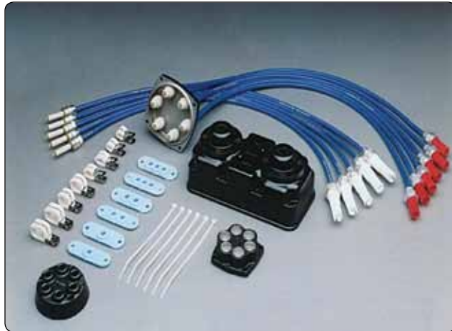
Figure 4-11. A high-tension ignition harness.
