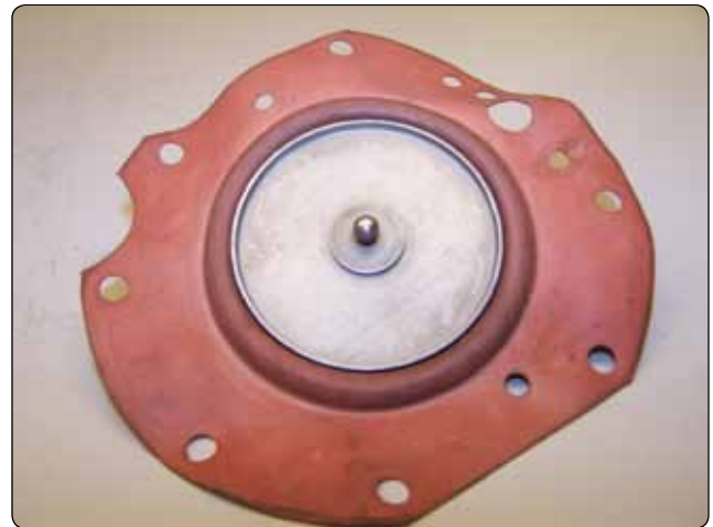
Figure 2-33. Fuel diaphragm with ball valve attached.
