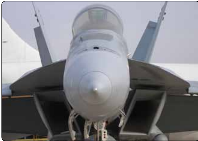
Figure 3-25. An example of a divided-entrance duct.
