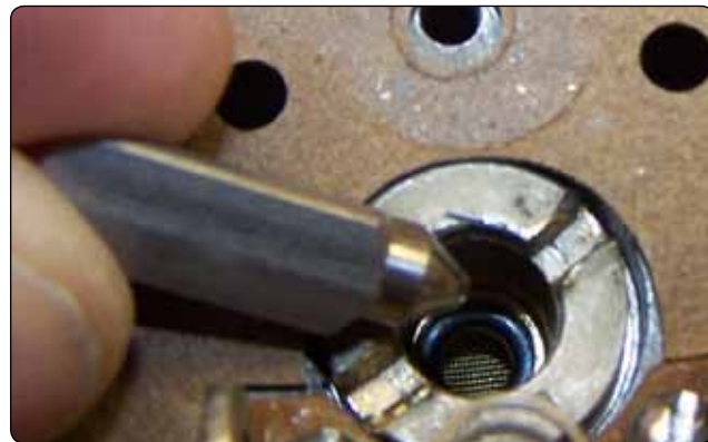
Figure 2-8. Needle valve and seat.
