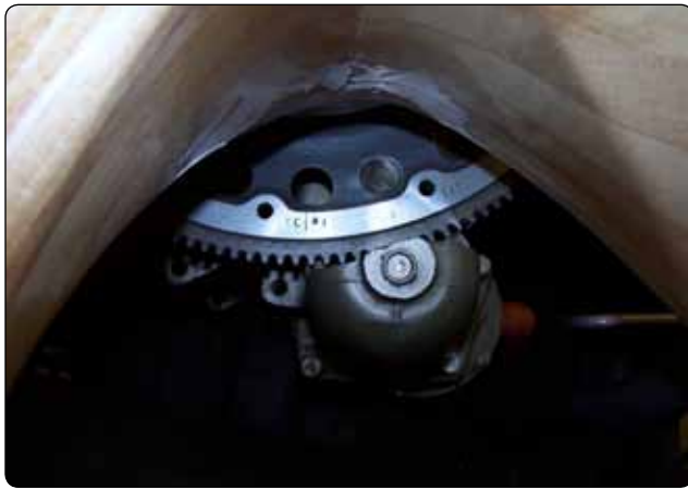
Figure 4-46. Timing marks aligned.
