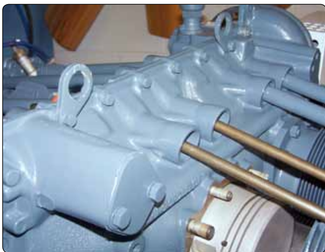
Figure 1-5. The crankcase.
