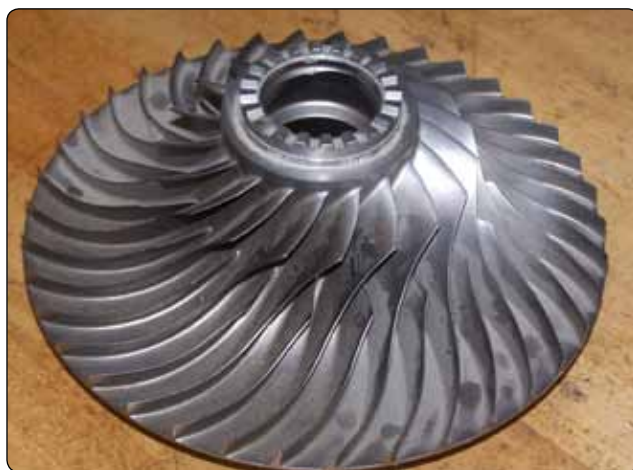
Figure 1-47. Single-entry impeller.
